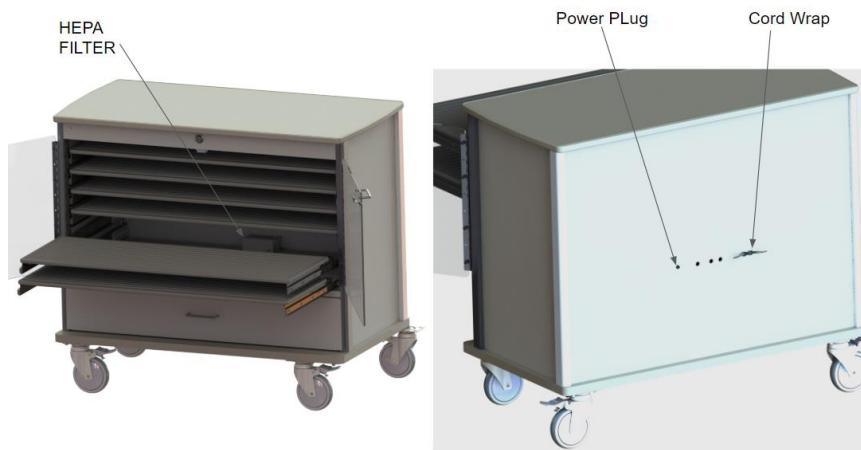
**Step 3:** Replace with new HEPA filter by sliding into box, keep the “grab tab” towards the outside for easy replacement next time.
