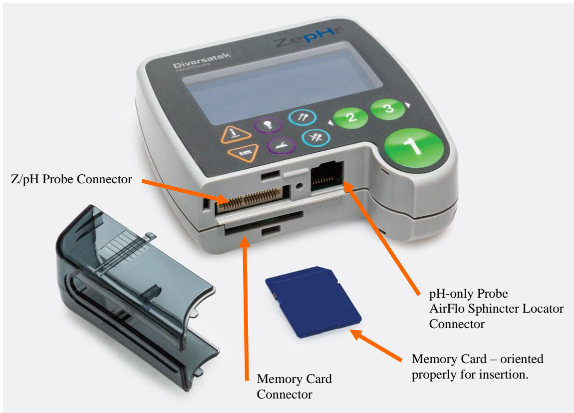
Figure 2: ZepHr Recorder - Top View with Cover Removed
