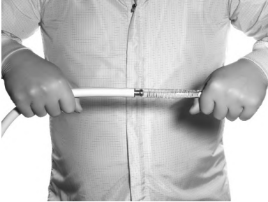
FIGURE 5. INCORRECT REMOVAL OF DETACHABLE TIP
