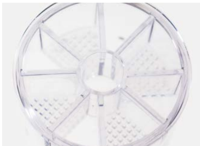
Four chambers with built-in strainers collect and separate specimens.
