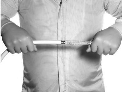
FIGURE 5. INCORRECT REMOVAL OF DETACHABLE TIP
