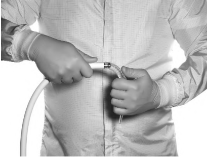
FIGURE 4. REMOVE THE DETACHABLE TIP WITH A PEELING MOTION
